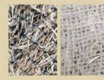
Aspen Excelsior Logs consist of a machineproduced high-altitude Rocky Mountain aspen excelsior matrix confined by a synthetic, tubular net to form a log of specific length, mass and diameter. Excel Aspen Excelsior Logs are designed to reduce hydraulic energy and filter sediment-laden flow in channels and on slopes. The logs are flexible, to conform to soil surfaces, and are secured by staking to create a temporary water-permeable structure.
