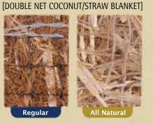
Excel CS-3 is an Extended-Term ECB comprised of a blended matrix of 70% certified weed free agricultural straw and 30% clean coconut. The blended matrix is mechanically (stitch) bound on two inch centers to Regular or All Natural netting. Excel CS-3 offers extended longevity, compared to straw matrix ECBs, thus providing a longer lasting alternative for moderate gradient slopes and channels.
